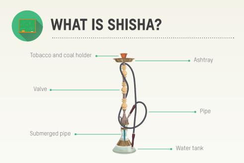
Shisha is a water pipe used to smoke tobamel heated with charcoal. At the top of the pipe, the tobamel is placed in the tobacco holder below the lit embers of coal. The smoker sucks into the pipe, which causes the smoke to flow down the immersed pipe. The smoke then rises to the surface of the water and then into the pipe.
